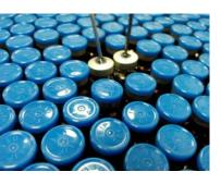
Rather than mounting externally like most sensors, our wireless data Loggers easily fits inside a variety of packages, like an ethylene oxide ER pack during sterilization, to maximize accuracy and process validation.
